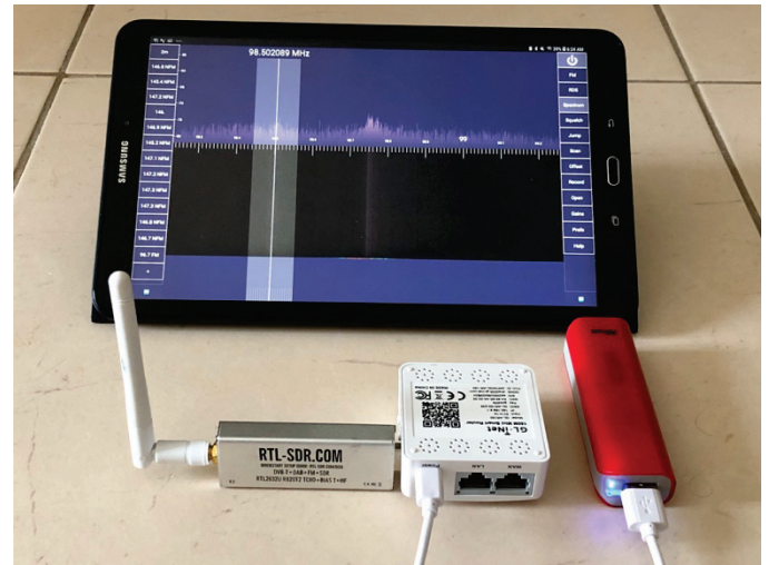
Fig. 14. No-Install RTL-SDR with Android, running SDR Touch Application.
