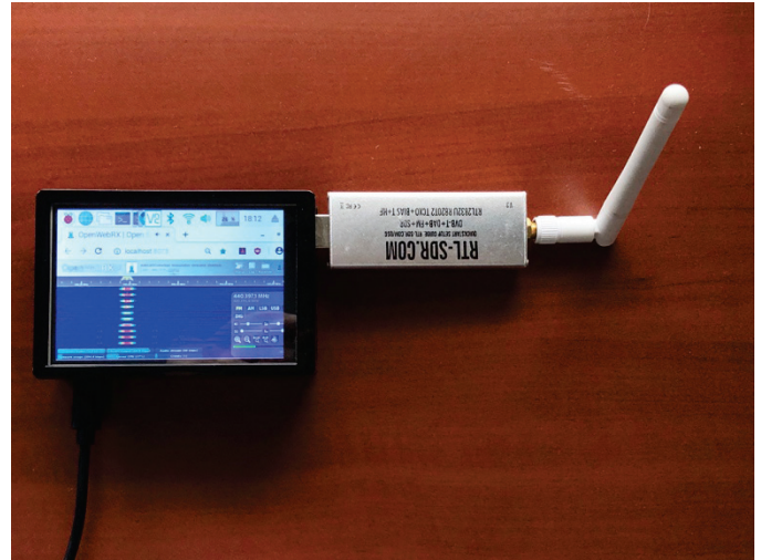
Fig. 12. Raspberry Pi Ground Station running OpenWebRX with Touch LCD Display
